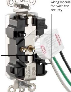
Nickel-plated brass single-piece wrap-around mounting strap with integral ground contacts for continuous conductivity and secure ground path (on select models) Two latches
